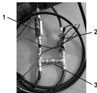
**Figure 5.** Hydraulic circuit supplemented by one-way valve: 1 – flowmeter on pressure branch (Q1), 2 – flowmeter on waste branch (Q2) with thermometer, 3 – one-way valve with spring.
