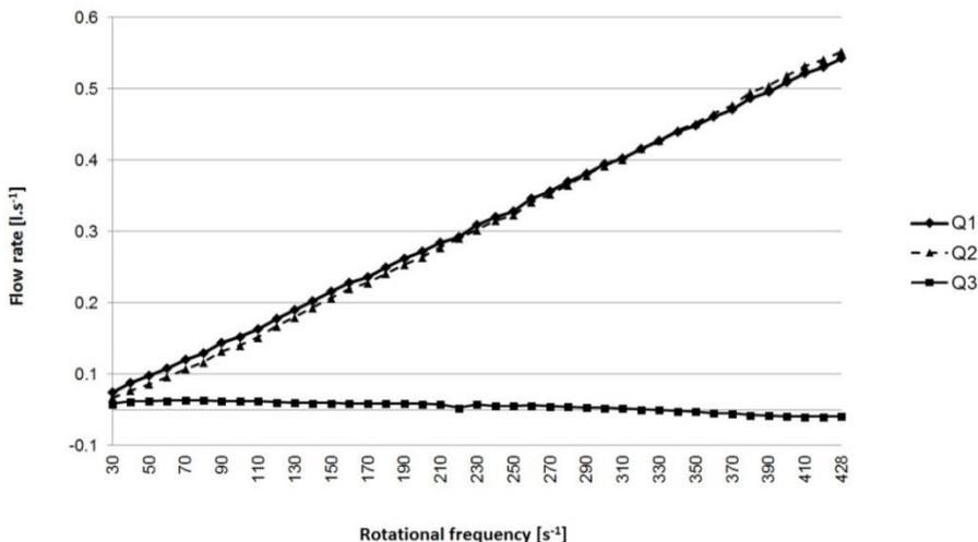
**Figure 7.** Graph of dependency of hydraulic oil flow on cutting disc rotational frequency: Q1 – hydraulic oil flow in pressure branch, Q2 – hydraulic oil flow in waste branch, Q3 – calculated flow of leakage fluid.
