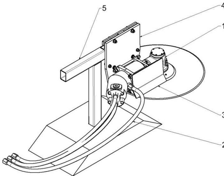
**Figure 3.** Laboratory set of mechanical pruner design: 1 – rear transmission with axial piston hydromotor, 2 – hydraulic lines, 3 – little plough blade, 4 – clamping plate, 5 – frame for laboratory measurement.
