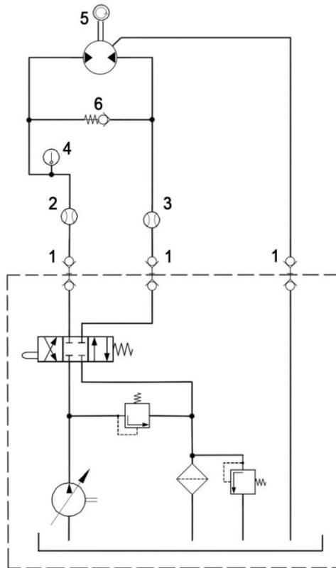
**Figure 6.** Designed hydraulic circuit: 1 – quick couplers, 2 – flowmeter on pressure branch, 3 – flowmeter on waste branch, 4 – thermometer, 5 – optical revolution counter of cutting disc, 6 – one-way valve with spring.
