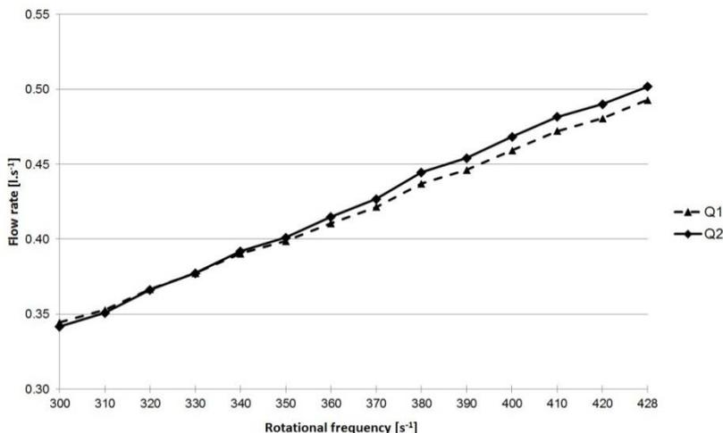
**Figure 8.** Detail of graph depicting dependency of hydraulic oil flow on cutting disc rotational frequency: Q1 – flow of hydraulic oil in pressure branch, Q2 – flow of hydraulic oil in waste branch.
