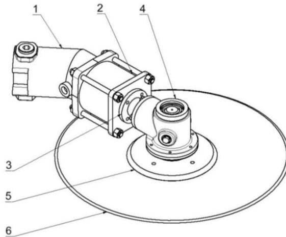
**Figure 2.** Rear transmission with hydromotor: 1 – axial piston hydromotor, 2 – coupler, 3 – extension, 4 – angular gear, 5 – carrier, 6 – cutting disc.
