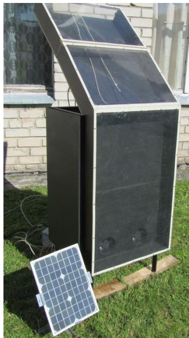
Figure 2. Autonomous, compact crop production drying facility.
