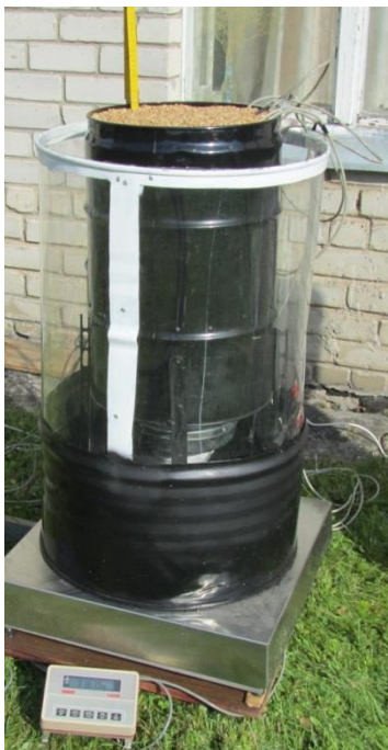
Figure 1. Cylindrical crop production drying device with solar collector.
