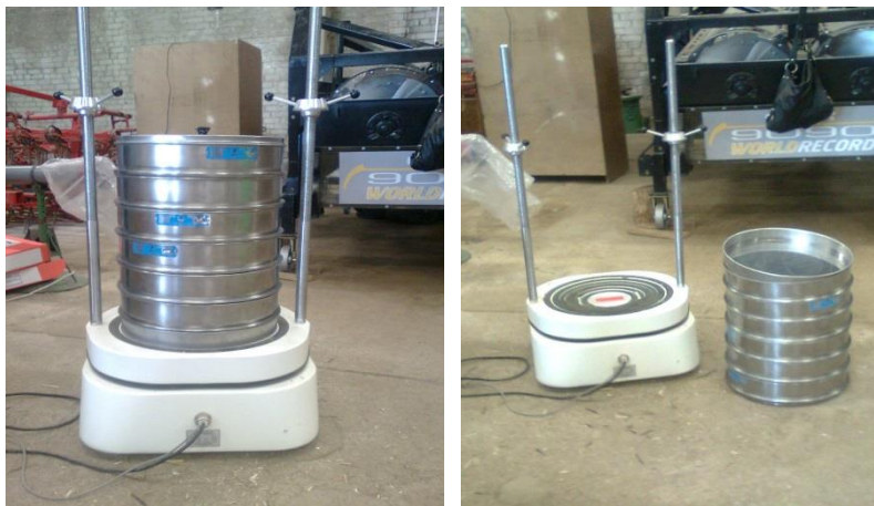
Figure 2. The stand for determination of chaff and flour fraction composition: vibratory device and sieves with the different diameter of holes.
