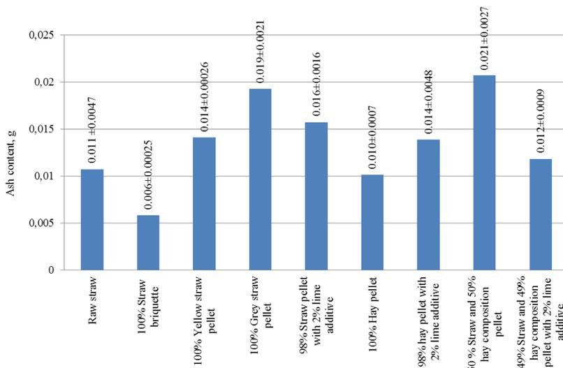
**Figure 2.** Ash content in tested samples.
