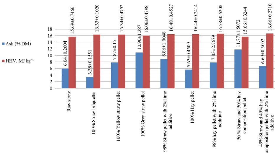
**Figure 3.** Ash amount and HHV in tested samples.
