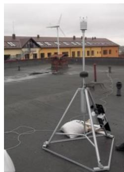
**Figure 3.** Vaisala weather station MAWS201 and 300 W wind generator.
