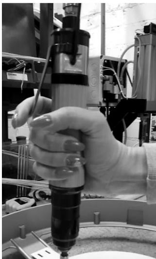
**Figure 2.** Pneumatic screwdriver.
