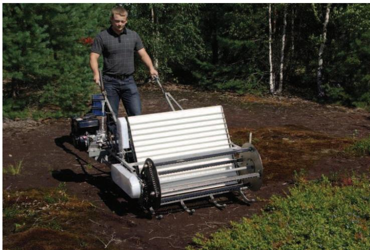
**Figure 3.** Prototype of the blueberry harvester.
