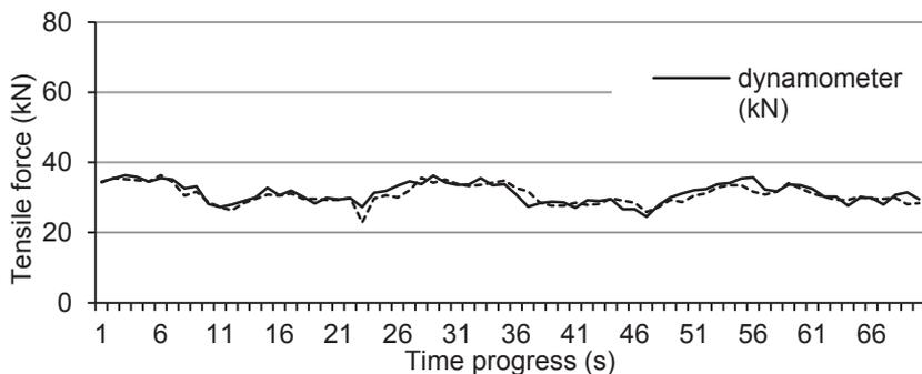
**Figure 3.** Time record of tensile forces measured with a tractor's in-built sensor and the dynamometer LUKAS type S-38 on plot No. 1.
