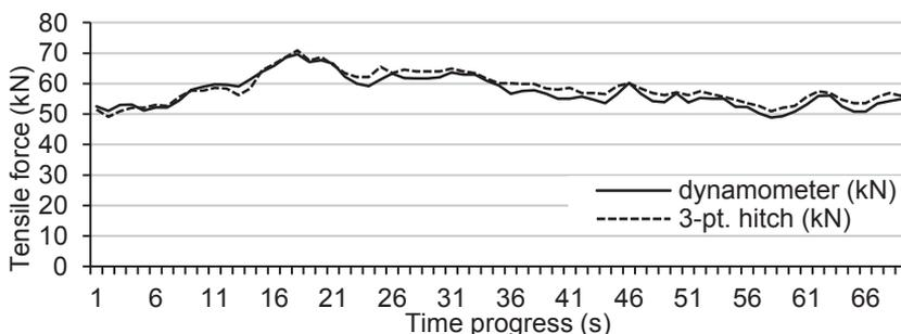
**Figure 4.** Time record of tensile forces measured with a tractor's in-built sensor and the dynamometer LUKAS type S-38 on field No. 2.
