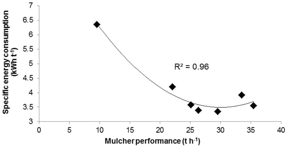
Figure 2. Specific energy consumption of the mulcher.
