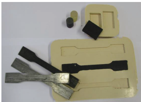
Figure 2. Models for forming, forms, test samples (for testing hardness, tensile strength, abrasive wear).
