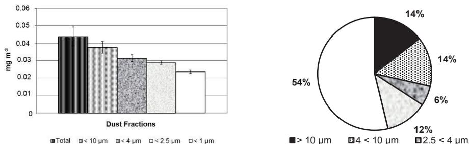
**Figure 3.** Concentrations and percentage of size distribution of dust fractions inside the office C.
