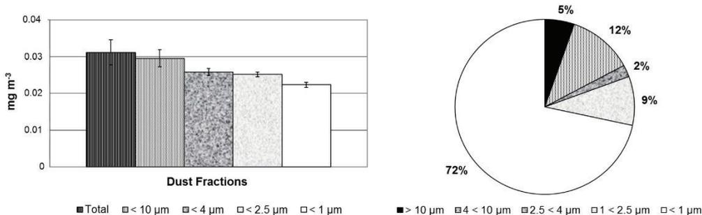
**Figure 4.** Concentrations and percentage of size distribution of dust fractions inside the office C after the wiping of the floor C<sub>2</sub>.
