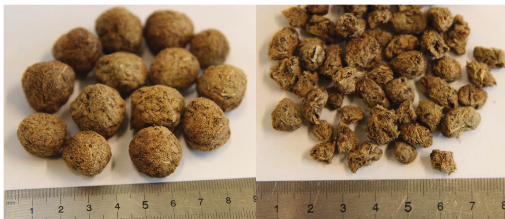
Figure 1. Samples of coniferous greenery granules (sample No. 1 on the left and sample No. 8 on the right).
