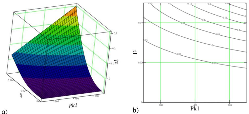
**Figure 5.** Surface (a) and profile graph (b) of function  $z_1 = z_1(P_1,t)$  for the transverse moving force variation within a range of  $P_1 = 100 \dots 700$  N ( $H = 500$  N,  $\nu = 10$  Hz).
