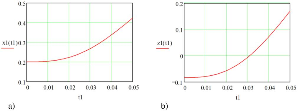
**Figure 2.** Graphs of the root's centre of mass displacement along the axes  $O_1x_1$  (a) and  $O_1z_1$  (b) as a function of time during the direct beet root lifting from the soil ( $H = 500$  N;  $P_1 = 400$  N;  $R_x = 100$  N;  $R_z = 100$  N;  $\nu = 10$  Hz).
