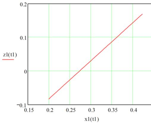
**Figure 3.** Beet root motion trajectory in the coordinate system  $x_1O_1z_1$  during the direct lifting of the root from the soil: ( $H = 500$  N,  $P_1 = 400$  N,  $R_x = 100$  N,  $R_z = 100$  N,  $\nu = 10$  Hz).
