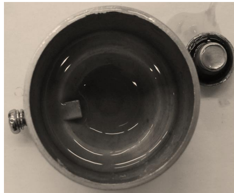
Figure 11. Accumulated oil in carburettor float chamber.
