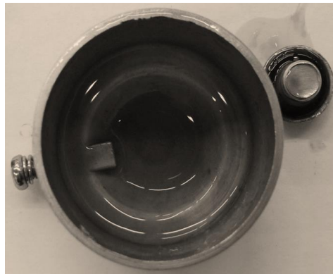
Figure 11. Accumulated oil in carburettor float chamber.
