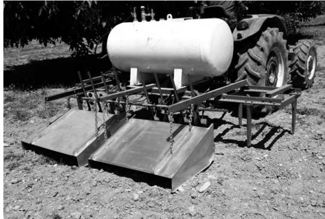
Figure 1. The weed flamer developed in this study.
