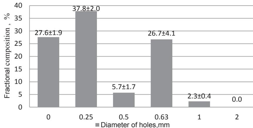
**Figure 2.** Fraction composition of fibre hemp Beniko mill.
