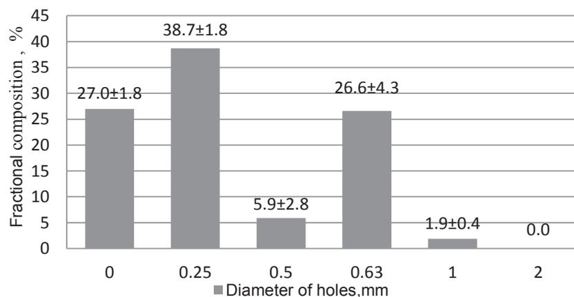
**Figure 3.** Fraction composition of fibre hemp Bialobrzeskie mill.
