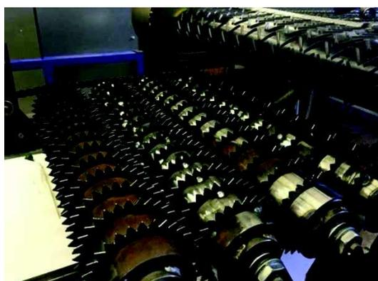
**Figure 2.** Laboratory roller conveyor with rollers fitted with welded collars with toothed profile.
