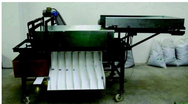
**Figure 1.** Model of a roller conveyor.
