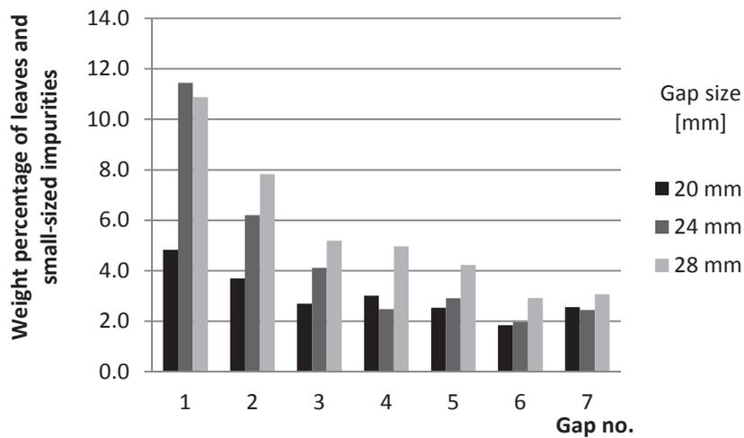
**Figure 6.** Weight percentage of the leaves and small-sized impurities fallen through the separate gaps for rollers of 89 mm in diameter and rotation frequency of  $0.67 \text{ s}^{-1}$ .
