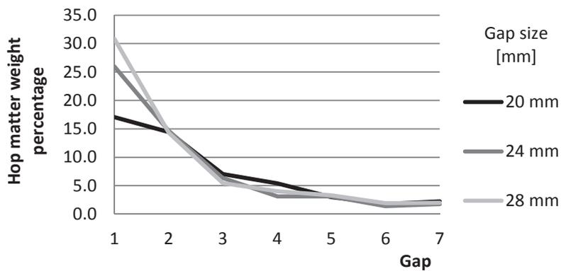
**Figure 4.** Weight percentage of the hop matter fallen through the separate gaps for rollers of 89 mm in diameter and rotation frequency of  $0.67 \text{ s}^{-1}$ .
