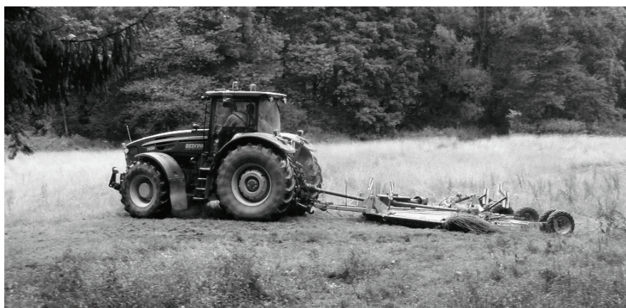
Figure 1. Working set of tractor John Deere 7930 and mulcher MZ 6000 during measurement.
