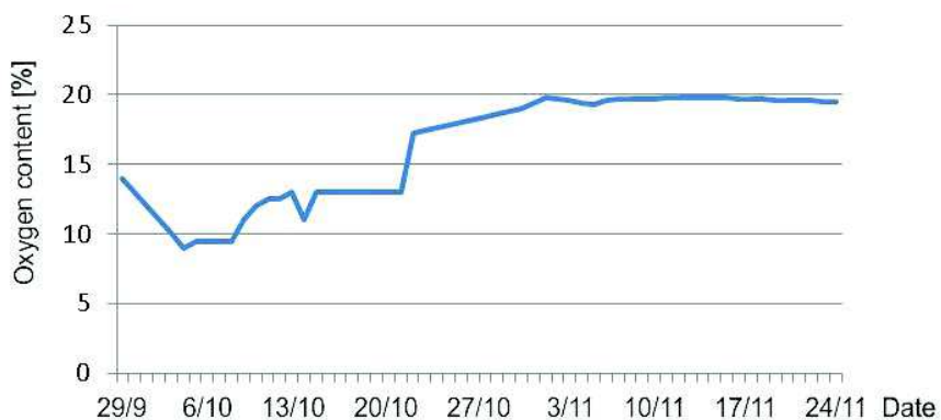
Figure 5. Measurements of the average oxygen content in the piles in autumn 2015.
