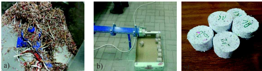
Figure 2. Briquette production process: a) a container with the material; b) conveyor of the briquettes; c) briquettes produced.
