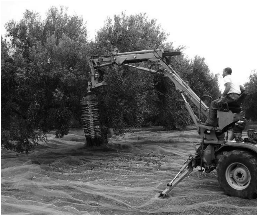
Figure 1. Mipe Viviani Oli-picker Olidb08 during harvesting trials.
