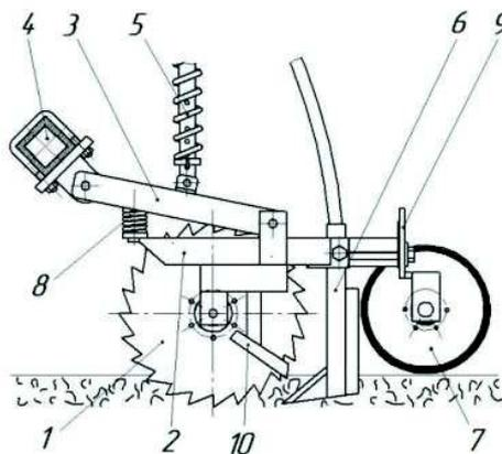
**Figure 1.** A scheme of combined opener assembly: 1 – toothed disc, 2 – spar, 3 – draw-bar, 4 – square beam, 5 – pressure spring, 6 – hoe-type seed conductor, 7 – packing wheel, 8 – spring assembly, 9 – adjustment device, 10 – cleaning device.
