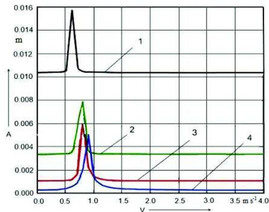
**Figure 3.** Curves of denoting the relation between the amplitude of vibration of opener assembly with a two-spring suspended toothed disc and the velocity of its motion at following deflection rates ( $\text{N m}^{-1}$ ):
