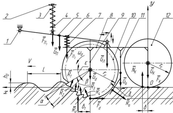
**Figure 2.** Theoretical schematic model of the improved design toothed disc opener assembly: 1 – breeding seed drill's draw-bar beam, 2 – pressure rod pivot journal, 3 – pressure spring, 4 – pressure rod, 5 – draw-bar, 6 – vibrator rod, 7 – vibrator spring, 8 – spar, 9 – rod, 10 – toothed disc, 11 – hoe-type seed conductor, 12 – packing wheel.
