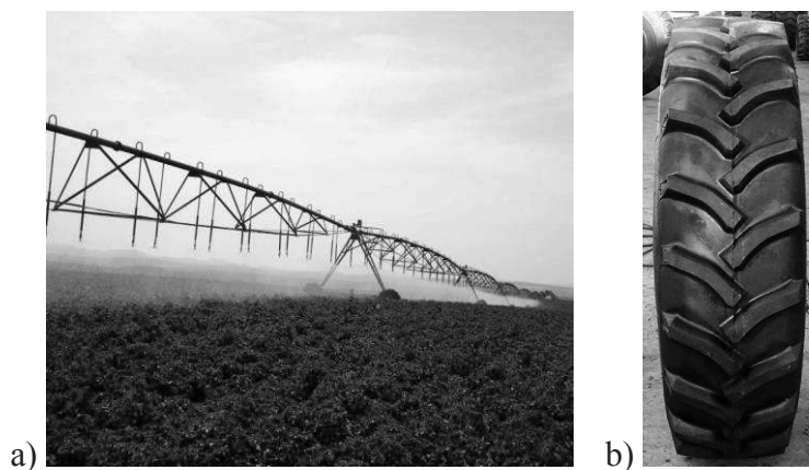
Figure 3. Linear irrigation machines (a) machine and (b) tyre, Valley Valmont, 600 m.
