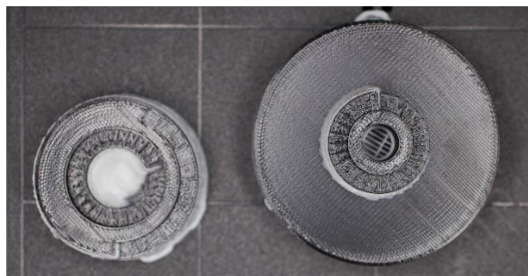
Figure 4. 2 nd generation 3D printed core and sleeve.
