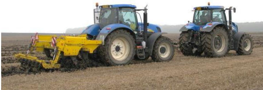
Figure 1. Photo of draft measurement of chisel plough Strom Terraland TN 3000 at Sloveč in autumn 2014.
