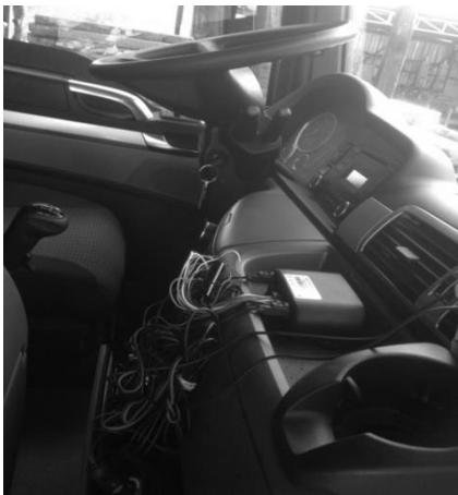
Figure 1. Installing the GPS/GSM black-box unit.
