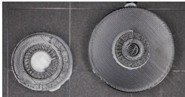
Figure 4. 2 nd generation 3D printed core and sleeve.
