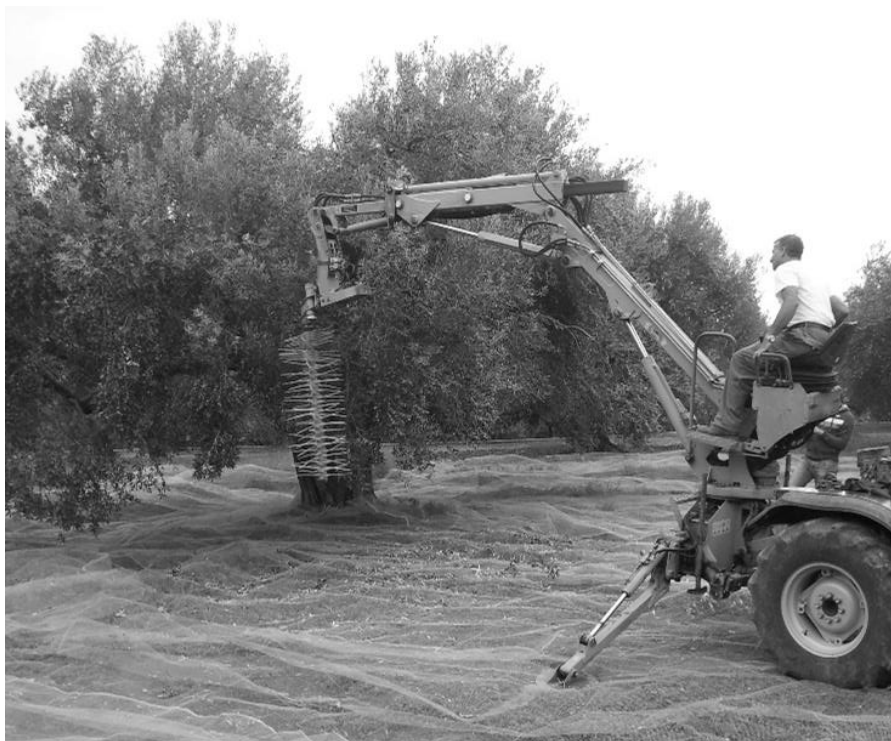
Figure 1. Mipe Viviani Oli-picker Olidb08 during harvesting trials.
