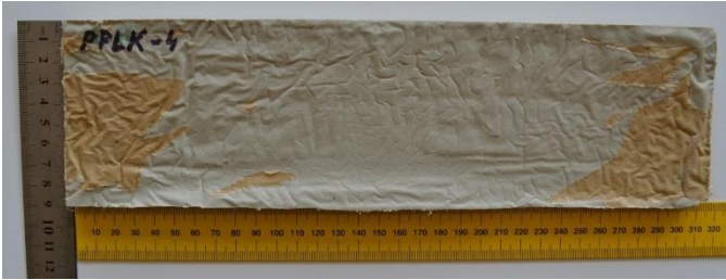
Figure 1. A composite polypropylene-perforated steel material – plane element.
