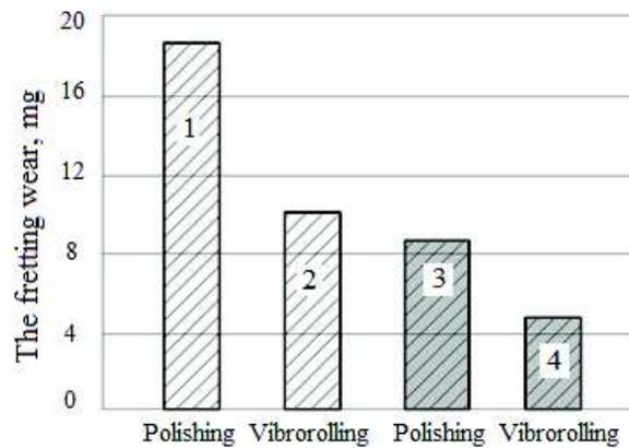
**Figure 6.** Fretting wear dependence on processing type: 1, 2 – steel samples and counter-samples; 3, 4 – cast iron samples, steel counter-samples; 1, 3 – after grinding; 2, 4 – after vibration knurling.
