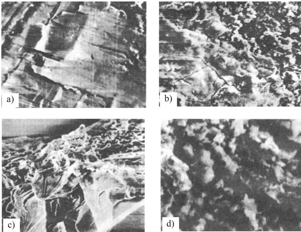
**Figure 5.** Fretting wear surface (friction mechanical brass plated steel): a) – a layer of brass plating on the friction surface (x 150); b) – alligatored brass plating after fretting (x 300); c) – transverse fracture surface of a plated sample in liquid nitrogen – loose porous brass coating on coarse grain steel base (x 400); d) – a fragment of low-temperature fracture of brass plating with a finely dispersed structure (x 7,000).
