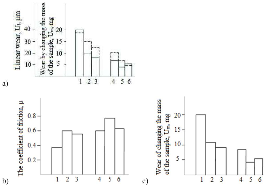
**Figure 2.** Fretting test results: a) – wear of samples (contour line – mass, dashed line – linear); b) – counter-samples wear; c) – established friction coefficient values; 1–3 – steel specimens: 1 – uncoated; 2 – friction mechanical brass plating, thickness 3–5  $\mu\text{m}$ ; 3 – fluorocarbon polymer compound, thickness 5  $\mu\text{m}$ ; 4–6 – cast iron samples: 4 – uncoated; 5 – friction mechanical brass plating; 6 – fluorocarbon polymer compound.
