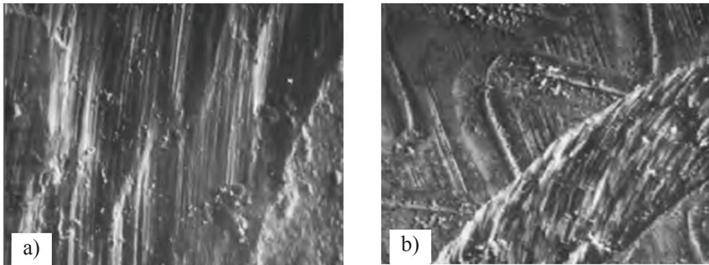
**Figure 7.** Fretting friction track on steel surface: a) – grinding; b) – vibration knurling.
