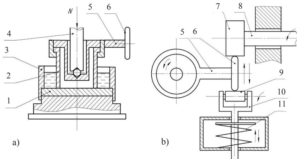
**Figure 1.** Friction machine FC: a) cross-section, b) top view: 1 – fixed sample, 2 – mobile sample, 3 – liquid process medium cell, 4 – thrust rod, 5 – rocker arm, 6 – roller; 7 – eccentric, 8 – drive shaft, 9 – pressure roller, 10 – fork, 11 – spring.
