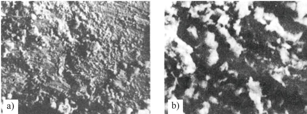
**Figure 4.** Fretting wear surface (fluorocarbon coated steel): a) – friction surface patch (x 200); b) – dispersed particles on friction surface, (x 2,000).
