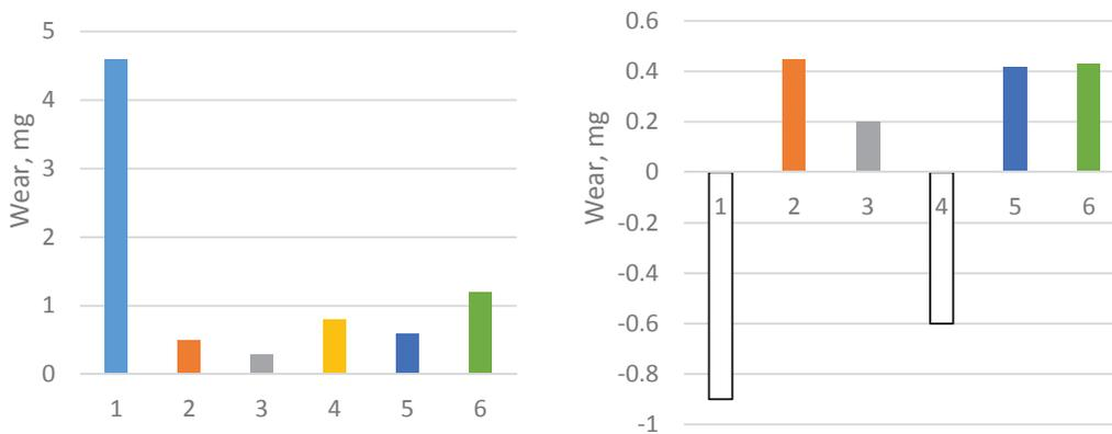
**Figure 9.** Wear of brass samples and counter-samples: 1 – unlubricated; 2 – VITREA 68 (SCHELL) oil; 3 – VITREA 68 (SCHELL) oil with 2.5% C<sub>60</sub>; 4 – ALVANIA EP2 (SCHELL) grease; 5 – ALVANIA EP2 (SCHELL) grease with 2.5% C<sub>60</sub>; 6 – C<sub>60</sub> coating on a brass sample, dry friction.
