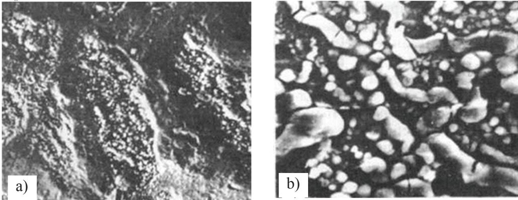
**Figure 3.** Fretting wear surface (steel): a) – caverns with wear particles, (x 160); b) – particles on the friction surface, (x 2,000).
