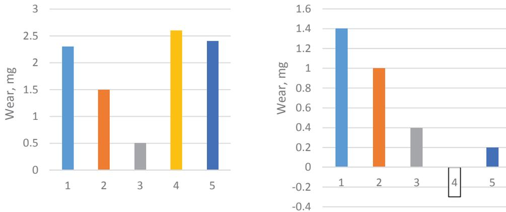
**Figure 8.** Wear of steel samples and counter-samples: 1 – unlubricated; 2 – VITREA 68 (SCHELL) oil; 3 – VITREA 68 (SCHELL) oil with 2.5% C<sub>60</sub>; 4 – ALVANIA EP2 (SCHELL) grease; 5 – ALVANIA EP2 (SCHELL) grease with 2.5% C<sub>60</sub>.
