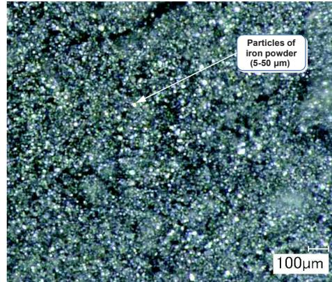
**Figure 7.** Iron powder particles after processing in disintegrator (Equipment: Keyence VHX-2000).
