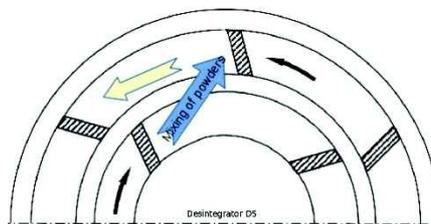
**Figure 3.** Multifunctional disintegrator: mixing process schematics (Tallinn University of Technology).
