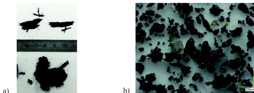
**Figure 4.** Optical microscopy of a crumb rubber before (a) and after (b) HPGR (Fig. 2) processing.
