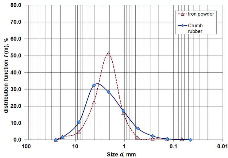
**Figure 5.** Crumb rubber and iron powder particles size distribution (Equipment: Analysette 22) used for feeding of multifunctional disintegrator (Processing stage 2, Fig. 1.).
