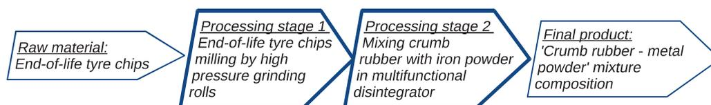
**Figure 1.** ELT rubber wastes transformation stages from tyre chips to 'Crumb rubber – metal powder' mixture composition.
