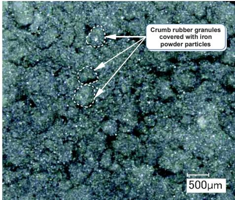
**Figure 6.** Crumb rubber granules covered with iron powder (Equipment: Keyence VHX-2000).
