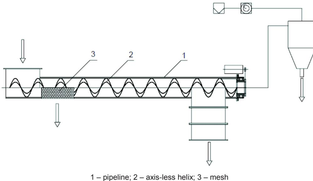
**Figure 1.** Schematic diagram of the spiral separator.
