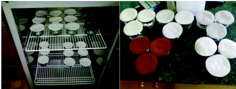
Figure 2. Test pieces sealed on vessels.
