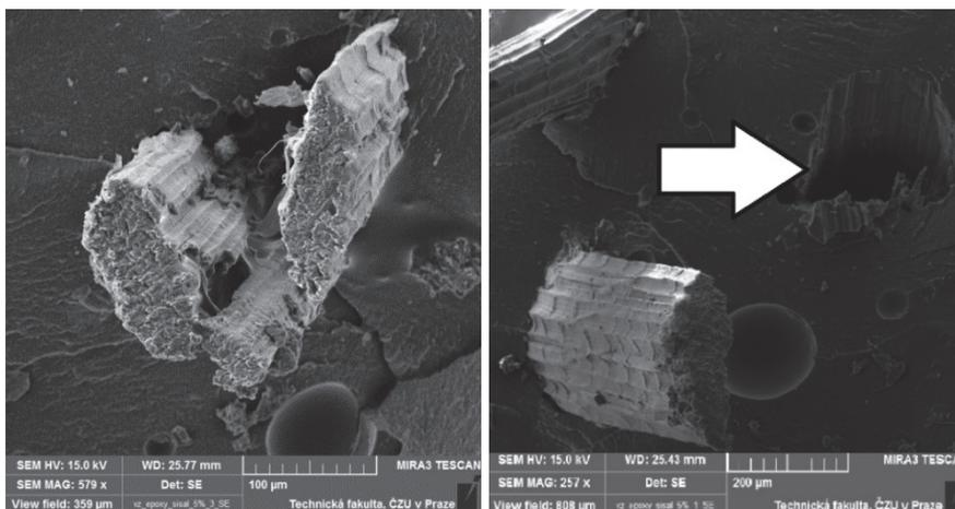
**Figure 5.** Fracture areas of sisal composites systems (SEM).
