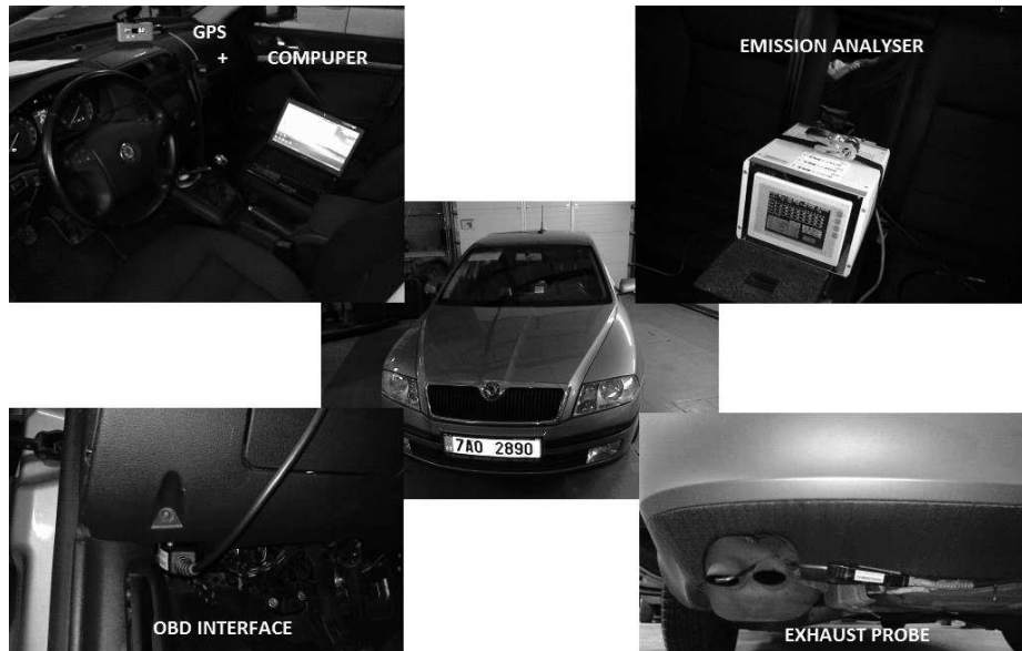
Figure 1. Equipment of measuring vehicle.
