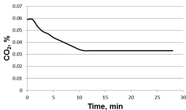
**Figure 2.** The course of  $CO_2$  concentration in the laboratory with level I of ventilation capacity.
