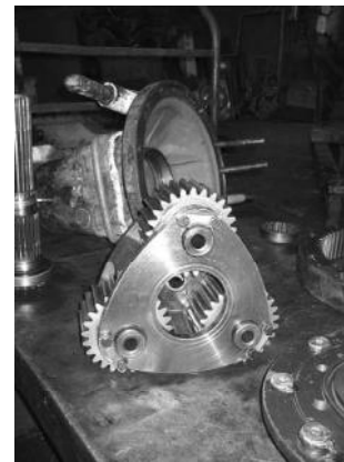
Figure 1. Tooth gear of end gear box (Aleš, 2009).
