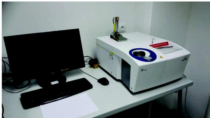
**Figure 1.** Mettler Toledo DSC unit.
