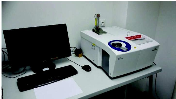
**Figure 1.** Mettler Toledo DSC unit.
