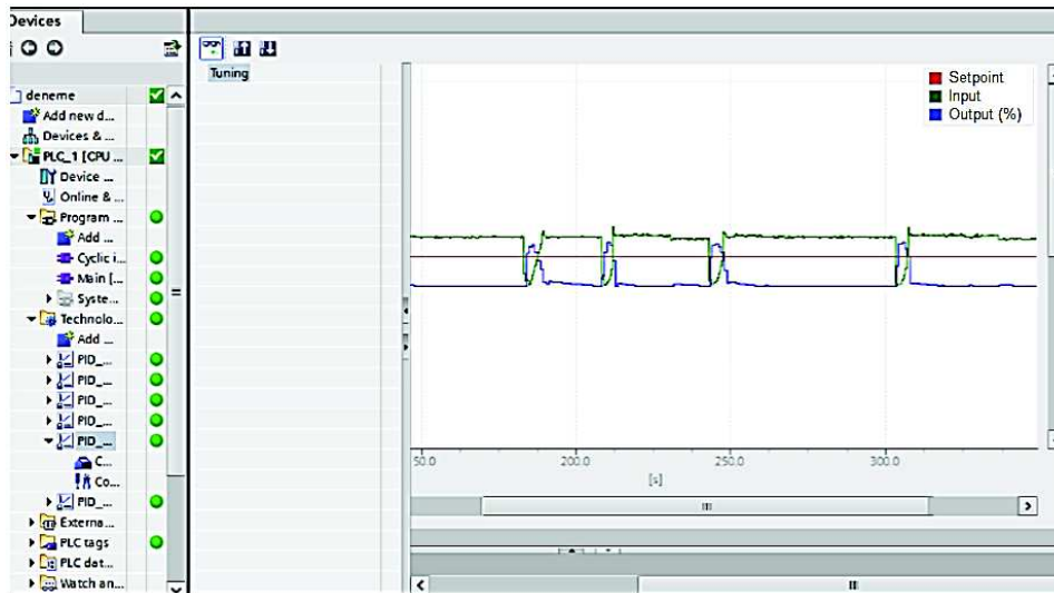
Figure 6. Tracking the set point, input, and output signals in an ongoing process.
