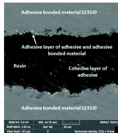
Figure 2. SEM images of cut through adhesive bond (MAG 2.02 kx).
