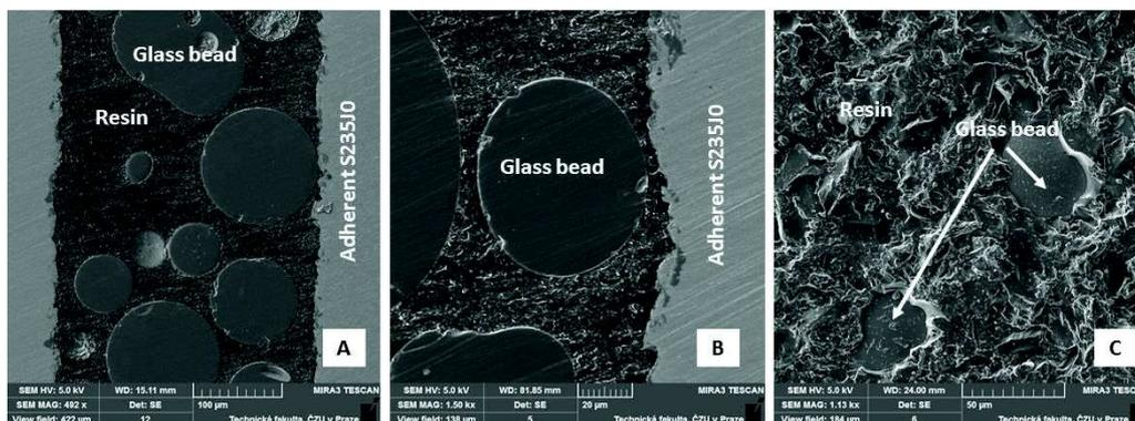
**Figure 6.** SEM images of cut through adhesive bond reinforced with glass beads (secondary electrons): A: cut through adhesive bond of resin reinforced with glass beads B 112 (MAG 492 x); B: good wettability of glass beads B 112 filler with resin (MAG 1.50 kx); C: adhesive – cohesive type of fracture surface of adhesive bond (MAG 1.13 kx).
