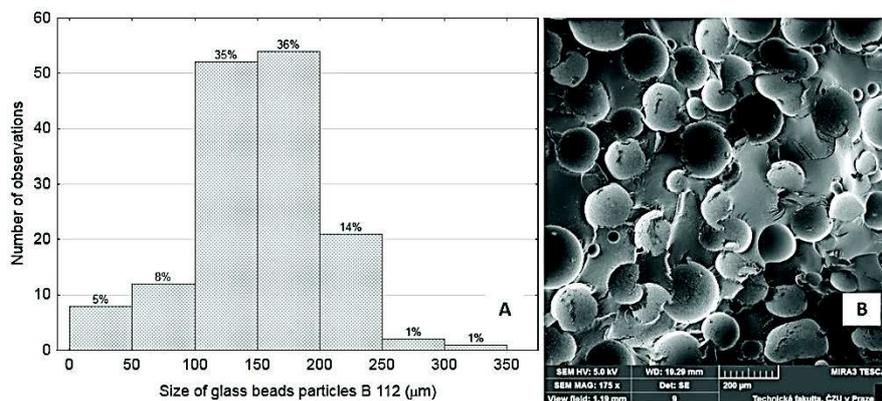
**Figure 1.** Filler in form of glass beads B112: A) Histogram, B) composite with spherical particles (SEM image, secondary electrons, MAG 175 x).
