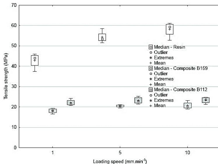
**Figure 3.** Influence of loading speed on tensile strength of resin and polymeric particle composite.
