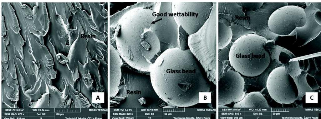
**Figure 4.** SEM images of fracture surface after tensile test (secondary electrons): A: Resin (MAG 675 x), B: interaction of resin and glass beads B112 (MAG 829 x), C: interaction of resin and glass beads B159 (MAG 829 x)
