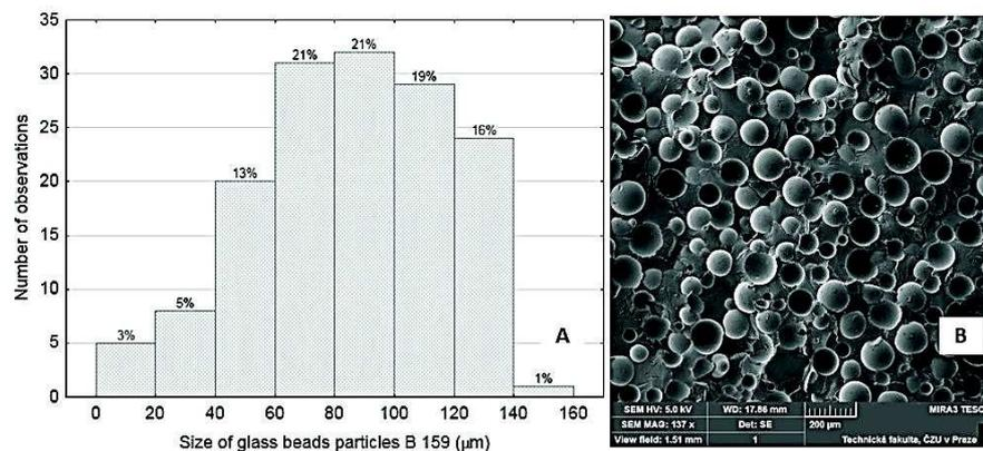
**Figure 2.** Filler in form of glass beads B159: A) Histogram, B) composite with spherical particles (SEM image, secondary electrons, MAG 137 x).
