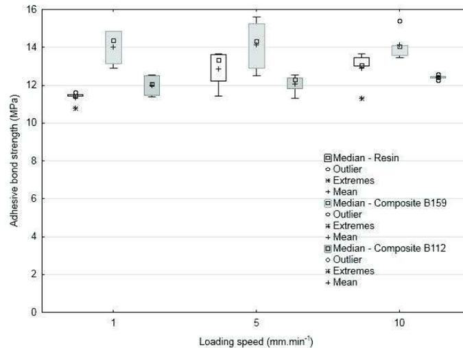
**Figure 5.** Influence of loading speed on adhesive bond strength of resin and polymer particle composite.
