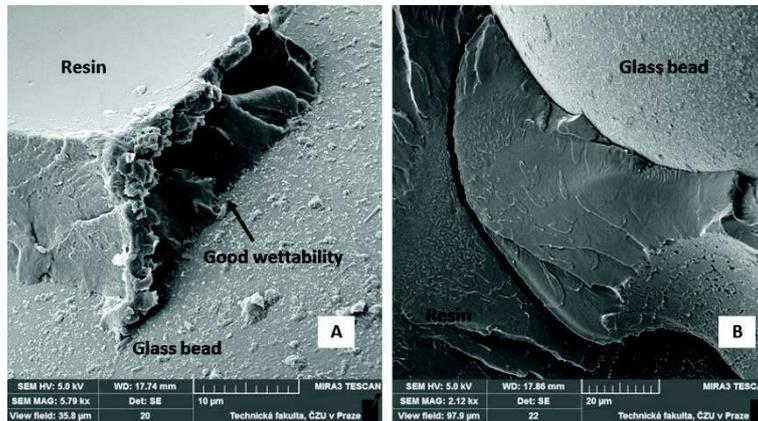
**Figure 7.** SEM images of fracture surface after shear tensile strength test of adhesive bonds (secondary electrons): A: good interaction of resin and glass beads B112, loading speed  $1 \text{ mm min}^{-1}$  (MAG 579 kx); B: fracture surface within adhesive layer stopped by glass beads B112 filler, loading speed  $10 \text{ mm min}^{-1}$  (MAG 212 kx).
