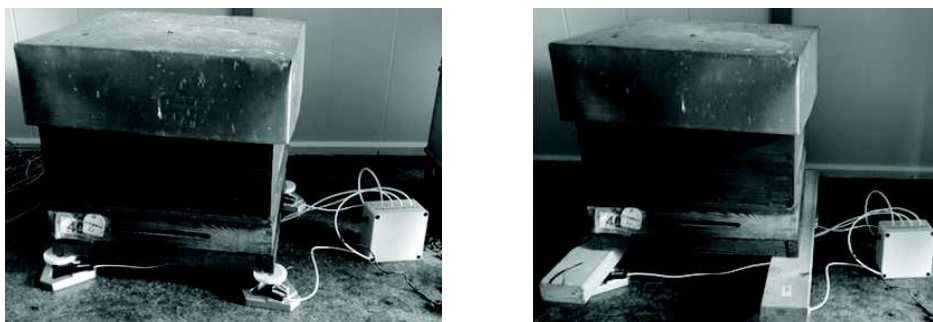
Figure 4. Installation of weight measurement system for beehive monitoring.
