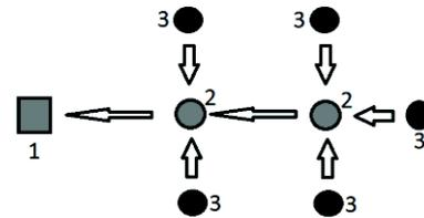
**Figure 2.** The transfer principle for a classic wireless network (1 – gateway; 2 – stationary repeater; 3 – transmitter).
