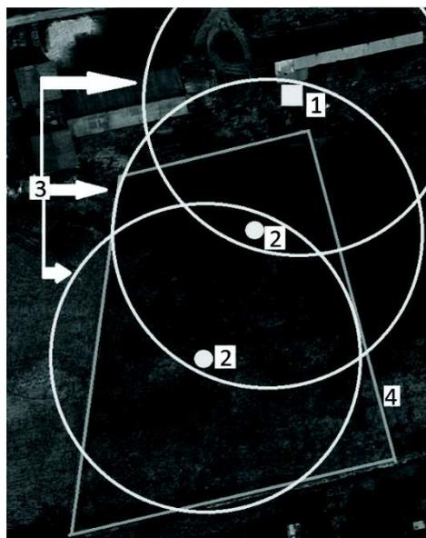
**Figure 3.** Design for a MESH wireless network distribution (1 – gateway; 2 – stationary repeater; 3 – wireless range, 4 – fence).
