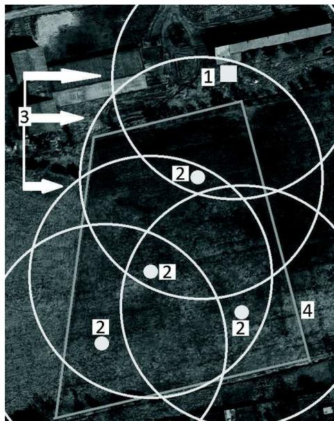
**Figure 1.** Design for wireless network distribution through stationary repeaters (1 – gateway; 2 – stationary repeater; 3 – wireless range, 4 – fence).
