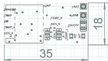
**Figure 7.** A printed circuit design for IQRF node connection for transmission of temperature.
