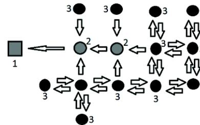
**Figure 4.** The transfer principle for a MESH wireless network (1 – gateway; 2 – stationary repeater; 3 – transmitter).
