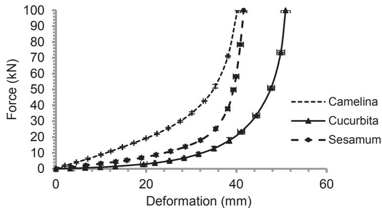
**Figure 2.** Measured mechanical characteristics of the selected oilseeds at pressing depths of 80 mm.
