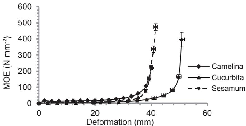
**Figure 4.** Moduli of elasticity of bulk camelina, pumpkin and sesame seeds gradually compressed to 100 kN.
