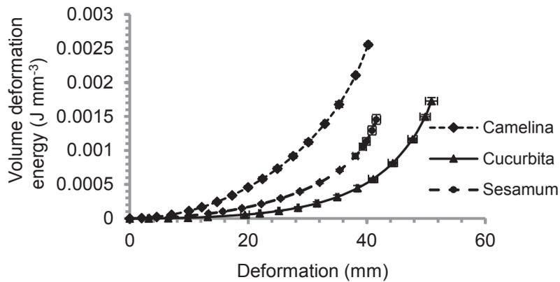
**Figure 3.** Changes in volume energy demands with incremental deformation of bulk camelina, pumpkin and sesame seeds loaded gradually to 100 kN.
