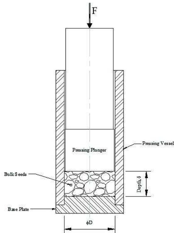
**Figure 1.** Schematic view of the oil expression apparatus.
