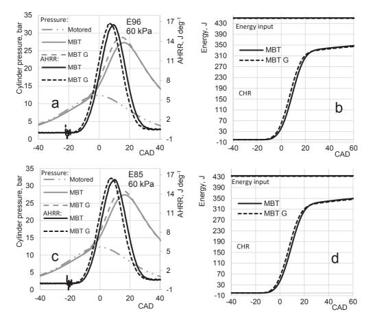
**Figure 6.** Cylinder pressure, apparent heat release rate and cumulative heat release, inlet manifold pressure 60 kPa. MBT – fuel's MBT timing, MBT G – gasoline MBT timing.
