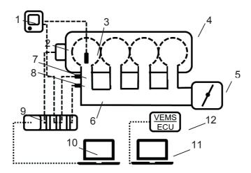
**Figure 1.** Cylinder pressure measurement setup: 1 – charge amplifier; 2 – crankshaft encoder; 3 – measuring spark plug; 4 – test engine; 5 – adjustable throttle valve; 6 – inlet manifold; 7 – inlet manifold pressure sensor; 8 – temperature sensor; 9 – data acquisition module; 10 – data acquisition control PC; 11 – ECU control PC; 12 – user controllable ECU.
