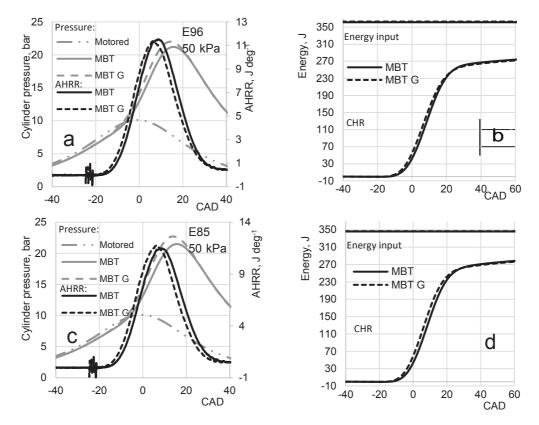
**Figure 5.** Cylinder pressure, apparent heat release rate and cumulative heat release, inlet manifold pressure 50 kPa. MBT – fuel's MBT timing, MBT G – gasoline MBT timing.
