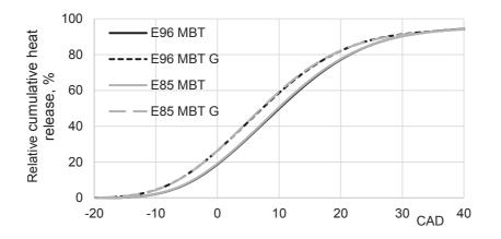
**Figure 2.** Relative cumulative heat release, engine speed 1,500 min<sup>-1</sup>, inlet manifold pressure 40 kPa, stoichiometric air/ fuel ratio.
