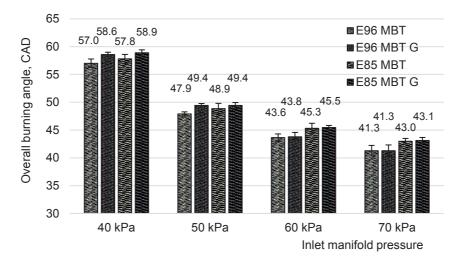
Figure 13. Overall burn angle at all test conditions.
