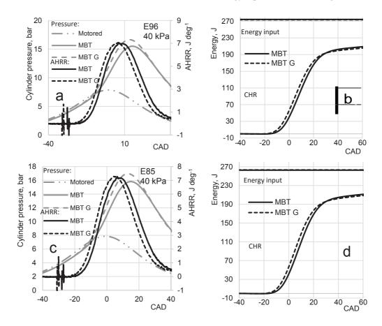
**Figure 4.** Cylinder pressure, apparent heat release rate and cumulative heat release, inlet manifold pressure 40 kPa. MBT – fuel's MBT timing, MBT G – gasoline MBT timing.
