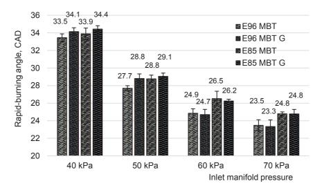
Figure 12. Rapid burn angle at all test conditions.
