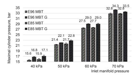
Figure 8. Maximal cylinder pressure at all test conditions.
