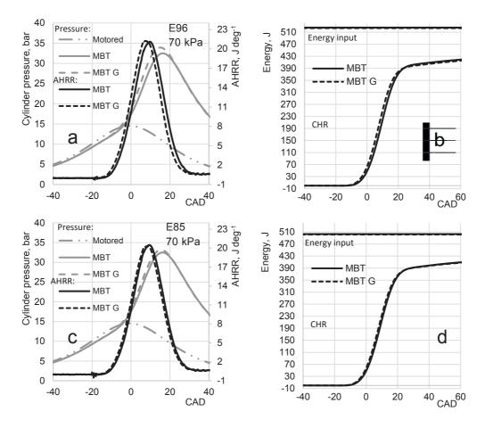
**Figure 7.** Cylinder pressure, apparent heat release rate and cumulative heat release, inlet manifold pressure70 kPa. MBT – fuel's MBT timing, MBT G – gasoline MBT timing.
