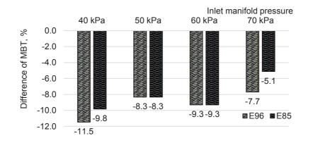
**Figure 3.** Relative difference of MBT advance, comparing to RON98 MBT, engine speed 1,500 min<sup>-1</sup>, stoichiometric air/ fuel ratio.
