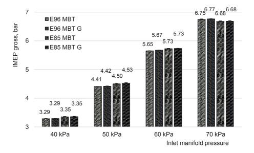
Figure 9. Gross indicated mean effective pressure at all test conditions.
