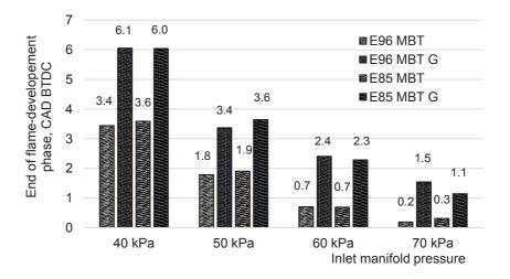
Figure 11. End of flame-development phase at all test conditions.
