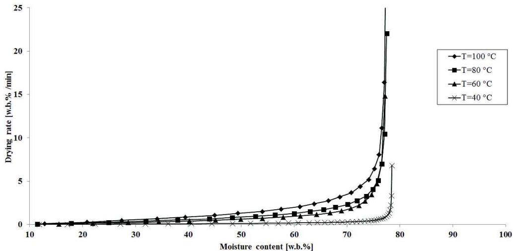
**Figure 3.** Drying rate versus moisture content at different air temperatures.
