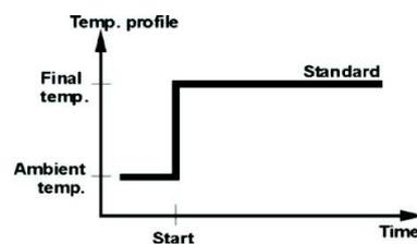
Figure 1. Drying profile: Standard for moisture balance Radwag
