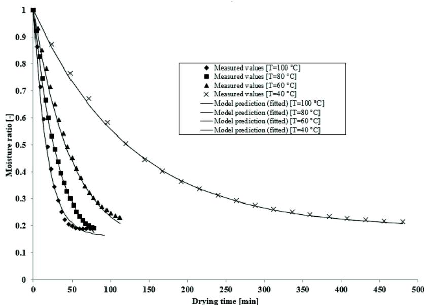
**Figure 2.** Comparison of measured values of moisture ratio and fitted models in the air temperature range of 40–100 °C.
