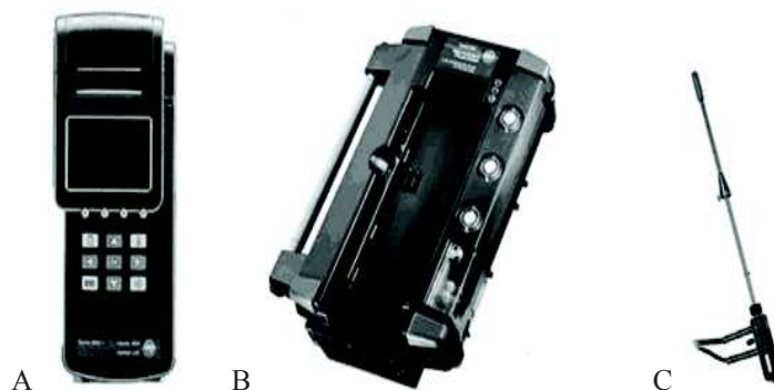
Figure 2. Modular system TESTO 350 M/XL for the analysis of flue gases: A – control unit; B – analyzer box; C – sampling probe.
