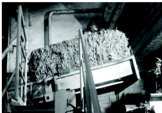
Figure 1. Package of maize cortical inserted into the dosing device of incinerator.
