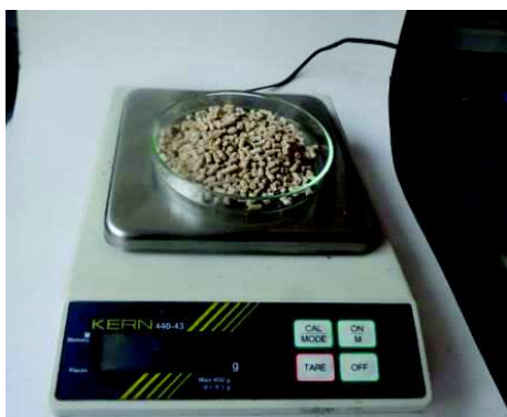
Figure 11. Weighing of 1,000 pellets made from pea with addition of 6% dried yeast.
