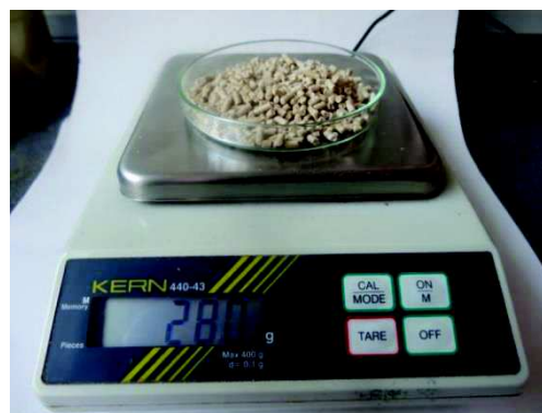
Figure 12. The weighing of 1,000 pellets, made from pea with addition of 6% dried yeast, diameter 3 mm, lengths 6,5 mm.
