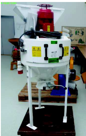
Figure 1. Vertical hammer mill type TAURUS.
