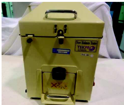
Figure 6. Picture of device for abrasiveness measurement New Holmen Tester TEK (general view).
