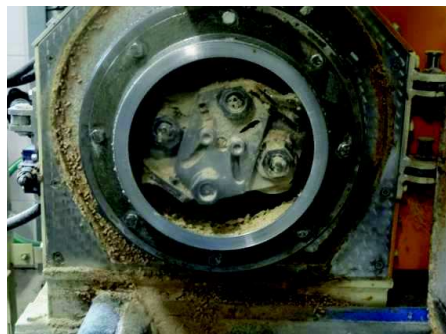
Figure 5. Picture of pellet press type Testmer 200, using the same matrix (wholes 3 mm).
