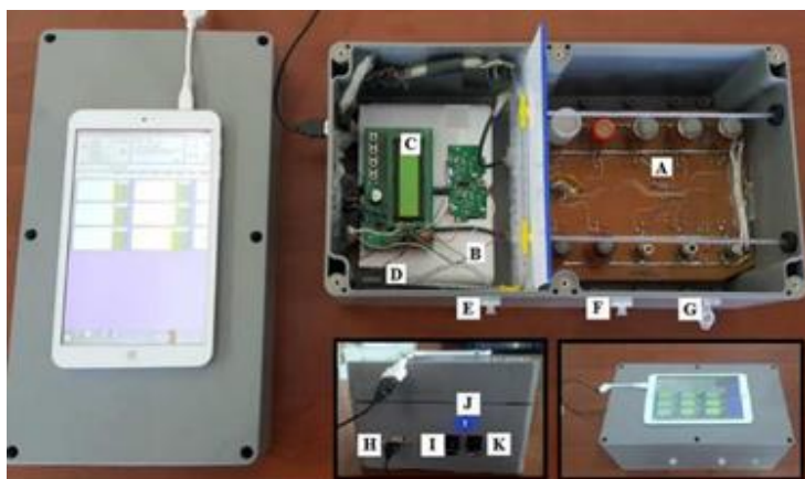
Figure 2. Modified e-nose system [A: sensor array, B: power bank, C: micro pump control unit, D: micro pump, E: sample air inlet, F: sample air outlet (reference gas inlet if needed), G: reference gas outlet (if needed), H: USB 4 port to tablet PC, I: sensor array power switch and USB charging port, J: power indicator LEDs, and K: micro pump power switch and USB charging port].
