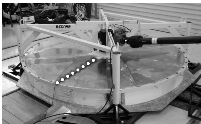
Figure 2. Laboratory model of one mulcher rotor with highlighted position of the pressure sensors by dotted line.
