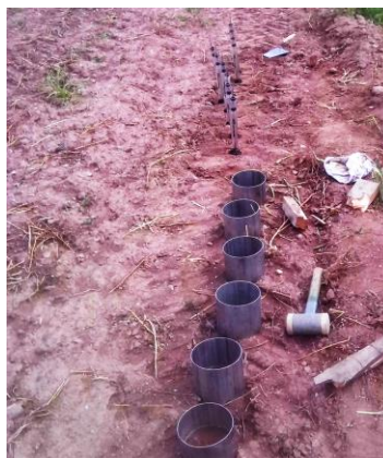
Figure 1. Measurements by Mini Disk infiltrometer and by Single Ring.
