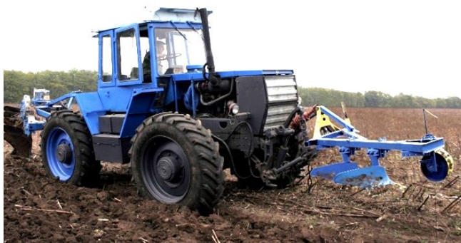
Figure 1. Tractor-implement unit operating on the 'push-pull' principle.
