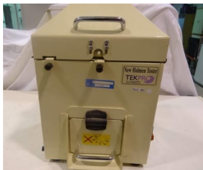
Figure 6. Picture of device for abrasiveness measurement New Holmen Tester TEK (general view).
