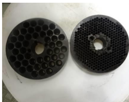
Figure 4. Matrix of pellet press JGE 120-6110 with wholes diameter 3 mm and 8 mm.
