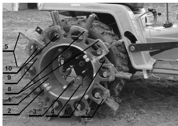
Figure 5. Blades wheel: 1 – support tube; 2 – locking tab; 3 – bracket fastening the mechanism to the wheel disc; 4 – spacer plates; 5 – blade; 6 – driving disc; 7 – blade control disc; 8 – guide pin; 9 – locking hole; 10 – blade pin; 11 – buffer plate.
