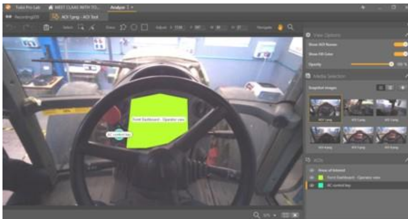
Figure 6. AOI1: the notification panel in the tractor dashboard and the Air conditioning rotary switch.
