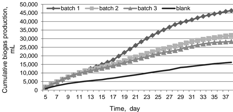
**Figure 3.** Cumulative biogas production of experimental batches.
