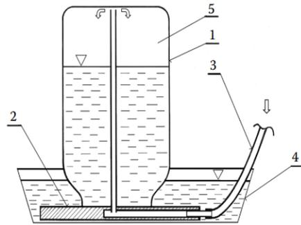
**Figure 2.** Equipment for measuring biogas volume based on water-column measuring system: 1 – glass jar; 2 – basic plate; 3 – biogas input; 4 – water basin; 5 – biogas produced.
