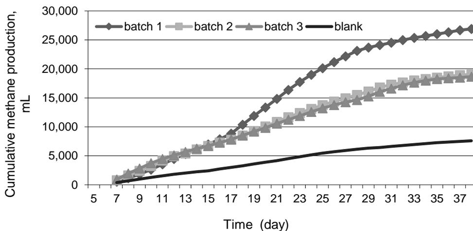
**Figure 4.** Cumulative methane production of experimental batches.
