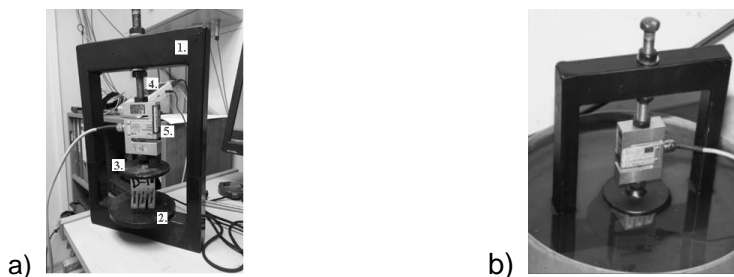
Figure 4. Swelling pressure measurement equipment with CWM sample in height direction (marked as D): a – sample before immersion in water; b – sample in a time of testing; 1 – frame; 2 – lower support; 3 – upper support; 4 –screw; 5 – load cell.
