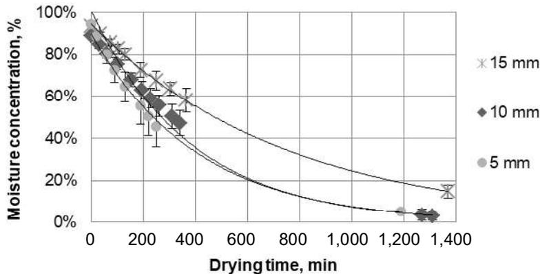
**Figure 4.** Average moisture concentration dependence on the drying time.
