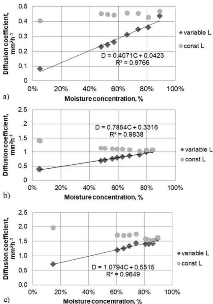
**Figure 6.** Diffusion coefficient dependence on the moisture concentration of slices taking and not taking into account the change in thickness during drying with: a) 5 mm thickness, b) 10 mm thickness, c) 15 mm thickness.
