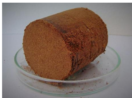
Figure 5. Produced bio-briquette sample before experimental testing.
