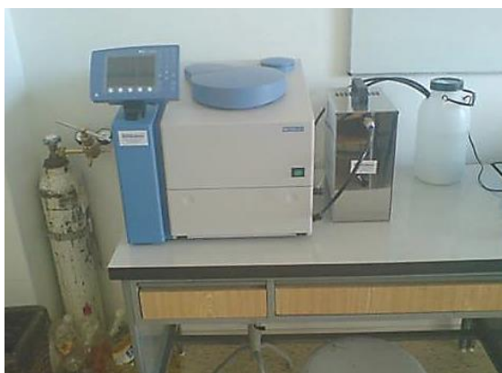
Figure 1. Calorimeter IKA C 6000 control unit (IKA® Works, Inc., USA).
